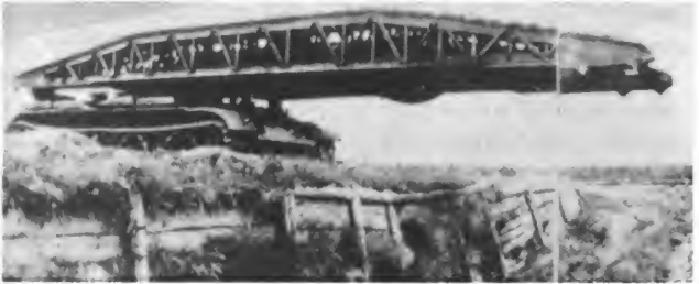
Figure 6-47. Tank-launched bridges. Two class-50 short-span bridges are used. The T-54 MTU (above) has a span of about 40 ft., while the (T-55) MTU-20 (below), with fold-up ramps at each end, has a span of about 68 feet.
